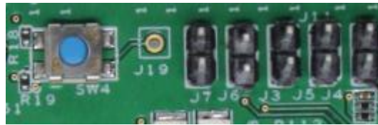
Figure 6: HW Control Signals Jumpers
